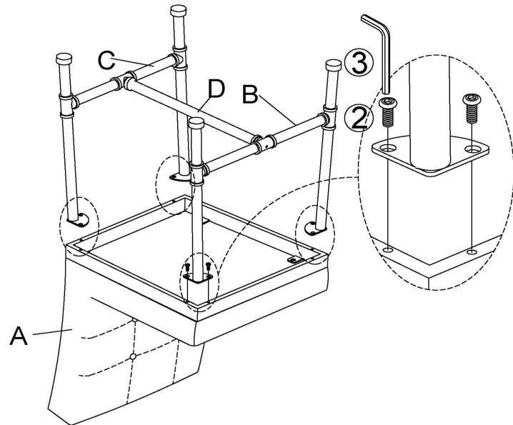
Attach Front leg(B), and Back Leg(C) to Seat(A) using Bolts(②) with Allen Wrench(③) as shown above.
