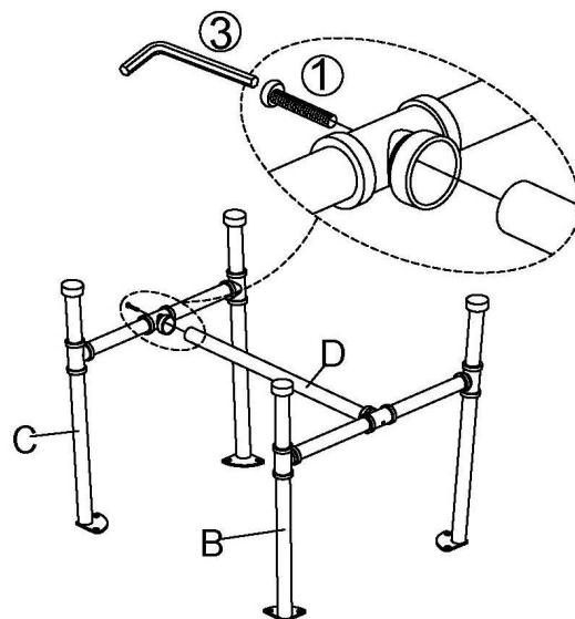
Attach Connecting Rod(D) to Back Leg(C) using Bolt(①) with Allen Wrench(③) as shown above.
