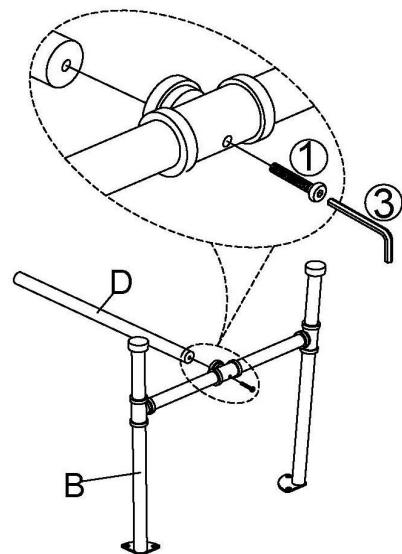
Attach Connecting Rod(D) to Front Leg(B) using Bolt(①) with Allen Wrench(③) as shown above.
